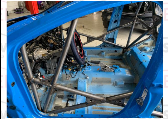
PHOTO 10 ANTI-INTRUSION DOORBAR - DRIVER
