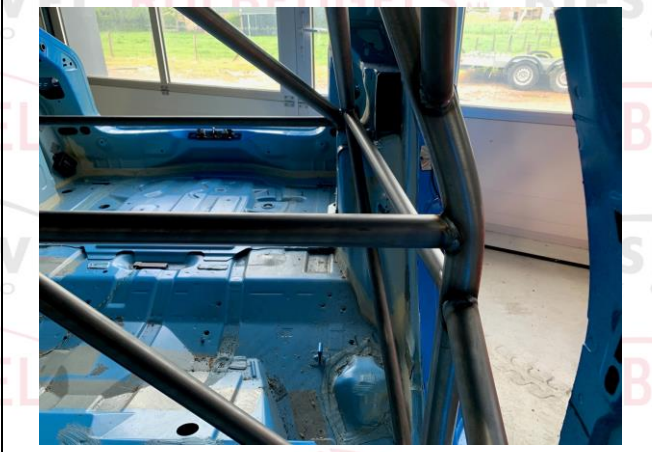
PHOTO 12 SHOULDER HARNESS ATTACHMENT - DRIVER
