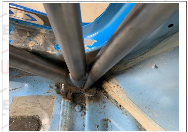
PHOTO 6 FRONT ROLLBAR TO FLOOR ATTACHMENT
